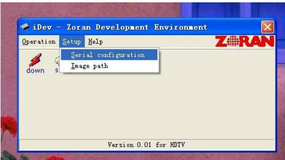
5. Confirm the Serial port is right. Base on the port which using for update. And set the band rate to 115200 (default).
